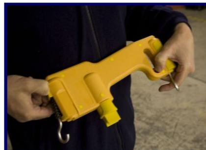
**6** Move the pointer towards the bottom of the scale (A) and push the spring assembly fully into the body (B).
