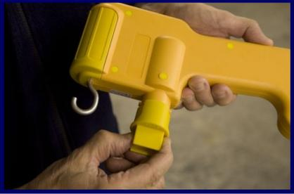
**9** Check that the end caps are correctly fitted by pushing firmly in the upward direction.
