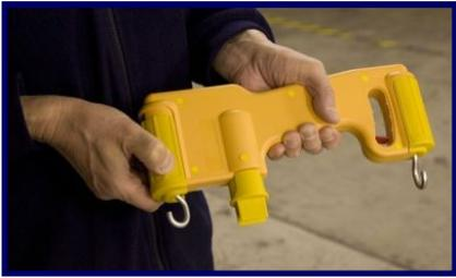
**8** Remove the rope locator by pulling it downwards. Refit correct rope locator.
