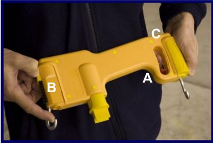
**7** Ensure that the hook bolt has the open end facing outwards and refit end cap.
